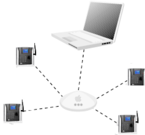
Ad-hoc (peer-to-peer) wireless network
